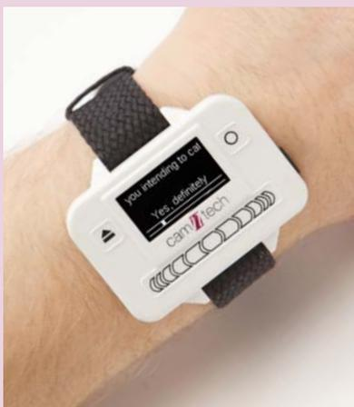
**The PRO-Diary** is a wrist-worn activity monitor with integrated Patient Recorded Outcome Diary. The diary user interface consists of a touch sensitive 'slider' device and two other buttons. It is designed to be easy to operate, and can ask questions of eight different types.
